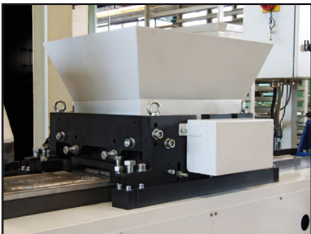
In the roof tile extrusion box DS-WFK, the roof tiles are formed. Our extrusion box is designed for extremely high pressures.
