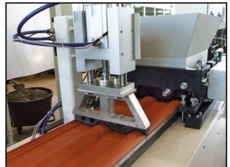
With the roof tile cutting station DS, the roof tiles are cut to roof tile length. The cutting blades are designed with radii, which form the frontal rounded edge of the roof tile.
